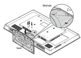
**3** Secure the stand with the three  $M4 \times L14$  mm screws (provided).
